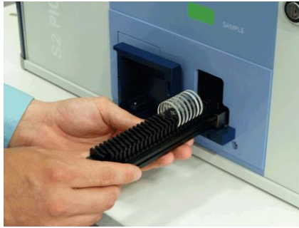
Figure 5. The sample insertion into the TXRF spectrometer
